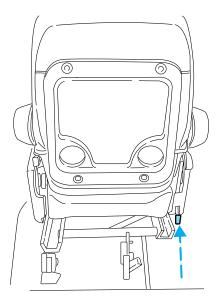
To return the seat to a seating position, move the seat rearward until the seat track locks. Then readjust the seatback.
